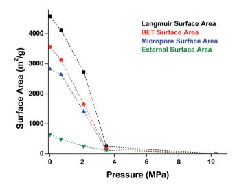
Fig. 5 Surface area of MOF-5 as a function of pressure. Elevated pressures were obtained using an anvil press in the absence of pressure transmitting fluid. Surface area values were determined using  $N_2$  adsorption measurements at 77 K. Adapted with permission from ref. 47. Copyright 2010 by American Physical Society.
