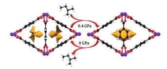
Fig. 9 Pore shape modification of  $Sc_2BDC_3$  upon exposure to 2-methylbutane at elevated pressure. Rotation of the phenyl rings reveals a larger cavity that can accommodate molecules that cannot fit in the pores at ambient conditions. Reprinted with permission from ref. 77. Copyright 2015, American Chemical Society.
