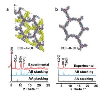
**Fig. 3** (a) The experimental PXRD and refined PXRD patterns, and the AB staggered stacking mode of COF-4-OH. (b) The experimental PXRD and refined PXRD patterns, and the AA eclipsed stacking mode of COF-0-OH.
