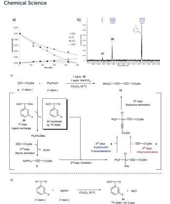
Fig. 4 Formation of "non-symmetric" I(iii) species by reaction of m-F-C<sub>6</sub>H<sub>4</sub> $I(OAc)_2$  **20** with Ph<sub>3</sub>PAuCl and methyl propiolate (5): (a) Evolution of the temporal concentration of reactants, intermediates and product. (b) <sup>19</sup>F NMR traces of the reaction mixture. (c) Rationalization of the observed species. (d) Alternative synthesis and characterization of m-F-C<sub>6</sub>H<sub>4</sub>I(OAc)(CI) (21).
