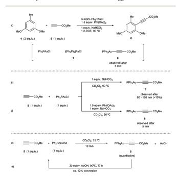
Fig. 2 (a) Standard catalytic reaction. (b and c) Experiments towards the formation of Au(ı)-acetylide 8 from Ph $_3$ PAuCl and alkyne 5 in the absence or presence of PhI(OAc) $_2$ , respectively. (d and e) Reactivity of Ph $_3$ PAuOAc towards methyl propiolate (5).
