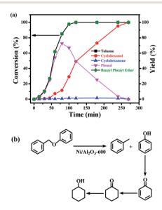
Fig. 5 (a) The time course of the product distributions for the conversion of benzyl phenyl ether ( $\alpha$ -O-4) over the Ni/Al<sub>2</sub>O<sub>3</sub>-600 catalyst. Reaction conditions: benzyl phenyl ether ( $\alpha$ -O-4) (185 mg, 1 mmol), Ni/Al<sub>2</sub>O<sub>3</sub>-600 (20 mg), solvent (10 mL), 150 °C, stirring at 1000 rpm. (b) Reaction pathway for the cleavage of benzyl phenyl ether.
