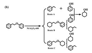
Fig. 7 (a) The time course of the product distributions for the conversion of 2-phenylethyl phenyl ether ( $\beta$ -O-4) over the Ni/Al<sub>2</sub>O<sub>3</sub>-600 catalyst. Reaction conditions: 2-phenylethyl phenyl ether ( $\beta$ -O-4) (198 mg, 1 mmol), Ni/Al<sub>2</sub>O<sub>3</sub>-600 (20 mg), solvent (10 mL), 170 °C, stirring at 1000 rpm, (b) reaction pathway for the cleavage of 2-phenylethyl phenyl ether.
