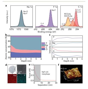
Fig. 2 Characterization of the in situ formed NaF-rich interphase on the surface of Na metal. (a) High-resolution XPS spectra of Na 1s, F 1s, and C 1s, (b) atomic percentages and (c) relative elemental intensities at different depths, (d) optical photograph, SEM image, and elemental maps (Na and F), (e) retracted force-distance curve, and (f) AFM topography image with a 3D view.
