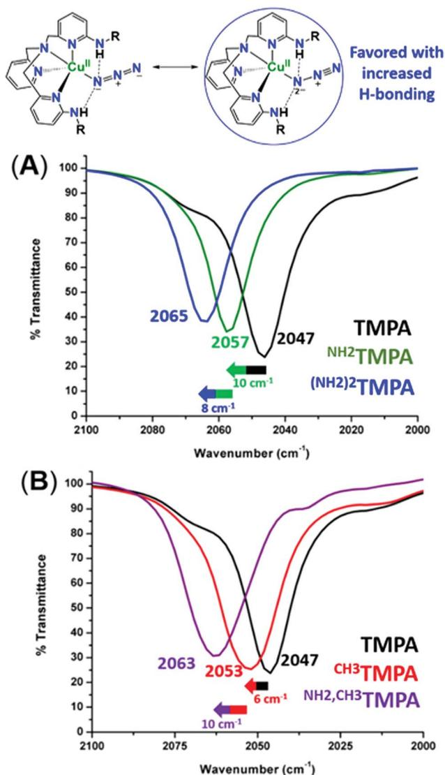
Fig. 3 Infrared spectra of  $[(^X\text{TMPA})\text{Cu}^{\text{II}}(\text{N}_3^-)]^+$  complexes in  $\text{CH}_3\text{CN}$ , showing the increase of the  $\nu(\text{N-N})$  stretch upon incorporation of amino substituents (A) and incorporation of steric functionalities (B).
