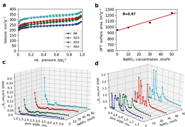
Fig. 5 (a)  $N_2$  sorption isotherms of all four samples, (b) correlation of DFT-derived surface area and  $NaNO_3$  content, (c) PSDs calculated by DFT (QSDFT (slit pore/cylindrical pore) model) based on the adsorption isotherms of  $N_2$  and (d) PSDs from  $CO_2$  adsorption (NLDFT, Non-Localized DFT method).
