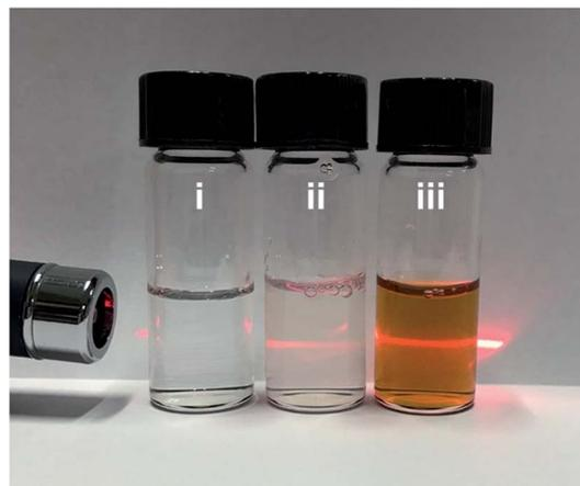
Fig. 2 Photo showing the Tyndall effect in solutions with different compositions: (i) PS-*b*-PEO dissolved in THF, (ii) PS-*b*-PEO dissolved in H<sub>2</sub>O mixed with 4% THF, and (iii) PS-*b*-PEO dissolved in H<sub>2</sub>O mixed with 4% THF + H<sub>2</sub>PdCl<sub>4</sub>.
