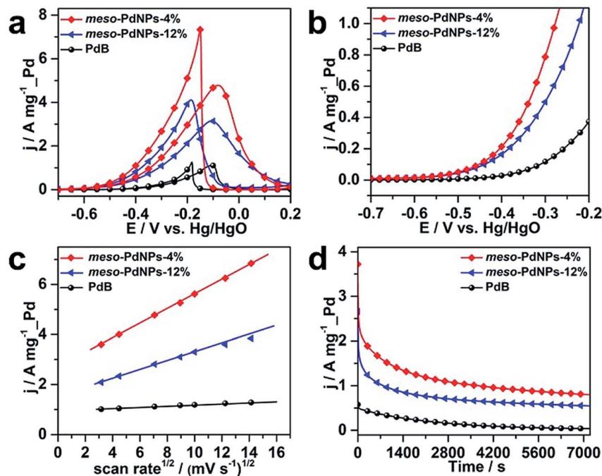
Fig. 6 (a) Mass-normalized cyclic voltammograms (CVs), (b) linear sweep voltammograms (LSVs), and (d) chronoamperometric curves (recorded at  $-0.2$  V) for EOR in  $1.0$  M NaOH containing  $1.0$  M  $C_2H_5OH$ . (c) The relationship of peak current density versus the square root of the scan rate. The CV and LSV curves were obtained at a scan rate of  $50$   $mV s^{-1}$  and  $1$   $mV s^{-1}$ , respectively.
