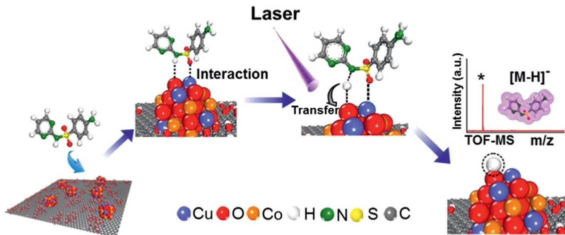
Fig. 6 Schematic diagram of the mechanism of SDZ ionization using the CuCoO-GO matrix for MALDI TOF mass spectrometry.
