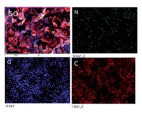
Fig. 2 Leucine functionalized graphene oxide elemental mapping.
