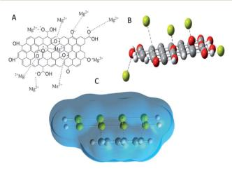
Fig. 10 Proposed mechanism: (A) suggested physisorption of negative charged functionalized GO materials on Mg alloy surface, (B) depiction of Mg<sup>2+</sup> state–alloy surface electrostatic interaction, (C) total electrostatic interaction of functionalized graphene oxide materials on Mg alloy.
