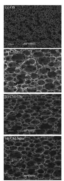
Fig. 5 Representative SEM micrographs (50 000× magnification; scale bar  $= 500 \, \mu m$ ) of the NR latex foam formed by (a) OS and (b) CM, and of the CM foam filled with either (c) USi or (d) MSi particles by different techniques.
