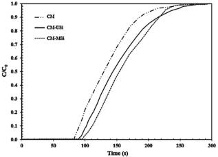
Fig. 8 Breakthrough curves of the NR latex foam, and the rubber composite of the CM foam filled with either USi (CM-USi) or MSi (CM-MSi) particles at a mixed gas flow rate of 100 mL  $\rm min^{-1}$  under ambient temperature and pressure.
