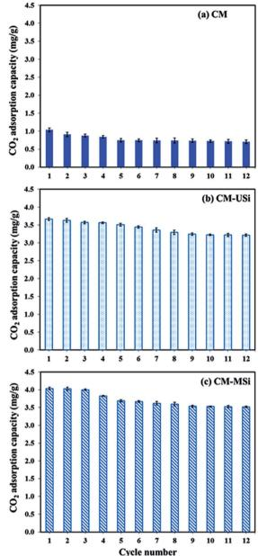
Fig. 9 The  $\rm CO_2$  uptake of (a) CM, (b) CM-USi and (c) CM-MSi foams over 12 adsorption–desorption cycles; adsorption: a mixed gas flow rate of 100 mL min<sup>-1</sup> under ambient temperature and pressure; desorption: 60 °C under vacuum for 20 min.
