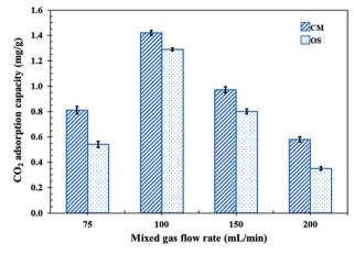
Fig. 6 CO<sub>2</sub> adsorption capacity of the CM and OS foams at different mixed gas flow rates (50, 75, 100, 150 and 200 mL min $^{-1}$ ) under ambient temperature and pressure.
