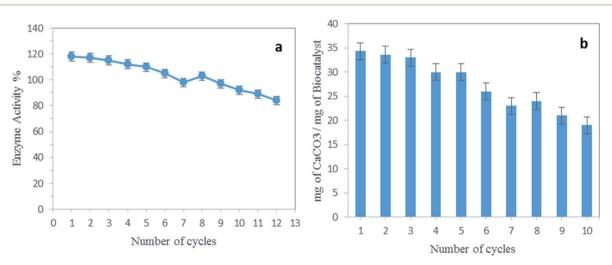
Fig. 8 (a) Reusability and (b) recyclability of the biocatalyst.
