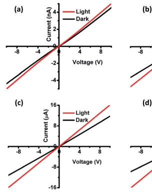
Fig. 8 Dark and light I-V characteristics of films (a) annealed at 350 °C, (b) selenized at 500 °C, (c) selenized at 525 °C and (d) selenized at 550 °C.
