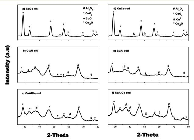
Fig. 3 X-ray diffraction patterns for calcined: (a), (b) and (c) and reduced Cu supported catalysts: (d), (e) and (f).
