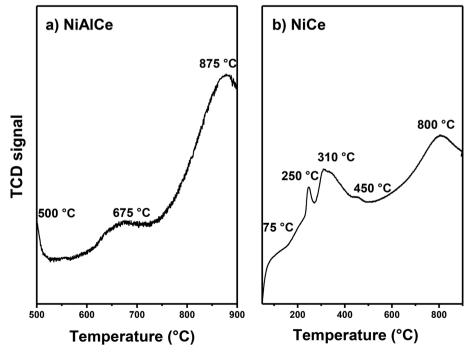
Fig. 12 H<sub>2</sub>-TPR profiles of calcined Ni NPS supported: (a) NiAlCe and (b) NiCe.
