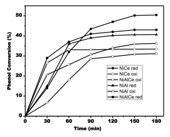
Fig. 15 Evolution of phenol conversion during single run catalytic tests for NiAlCe oxi ( $\square$ ), NiAlCe red ( $\blacksquare$ ), NiAl oxi ( $\triangle$ ), NiAl red ( $\blacktriangle$ ), NiCe oxi ( $\bigcirc$ ), NiCe red ( $\blacksquare$ ).
