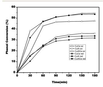
Fig. 13 Evolution of phenol conversion during single run catalytic tests for CuCe oxi  $(\triangle)$ , CuCe red  $(\blacktriangle)$ , CuAl oxi  $(\bigcirc)$ , CuAl red  $(\blacksquare)$ , CuAlCe oxi  $(\square)$ , CuAlCe red  $(\blacksquare)$ .
