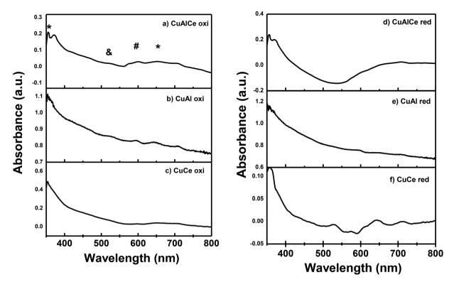
Fig. 5 Spectra UV-Vis for the calcined Cu supported catalysts: (a), (b) and (c) and, for the reduced Cu supported catalysts: (d), (e) and (f). Legend: (&) Cu<sub>2</sub>O, (#) CuO, (\*) Cu<sup>+2</sup> (Oh).
