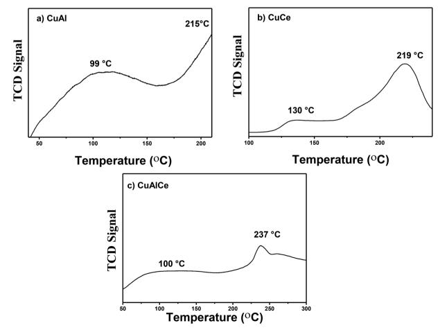
Fig. 11 H<sub>2</sub>-TPR profiles of calcined Cu NPS supported: (a) CuAl, (b) CuCe and (c) CuAlCe.
