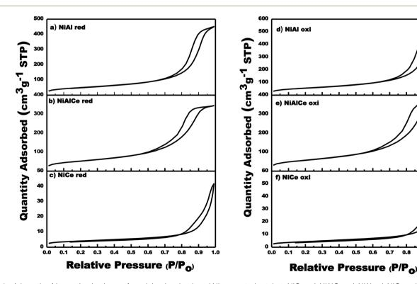
Fig. 2 Adsorption/desorption isotherms for calcined and reduced Ni supported catalyst: NiCe oxi, NiAlCe oxi, NiAl oxi, NiCe red, NiAlCe red and NiAl red.
