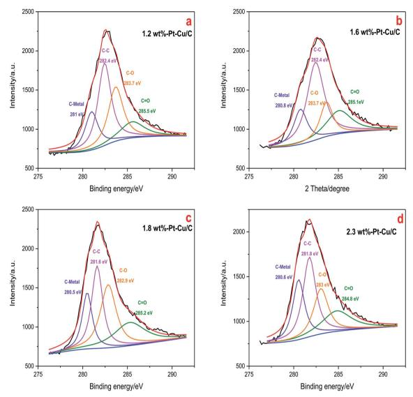
C 1 s XPS spectra of 1.2 wt% Pt-Cu/C catalyst (a), 1.6 wt% Pt-Cu/C catalyst (b), 1.8 wt% Pt-Cu/C catalyst (c), 2.3 wt% Pt-Cu/C catalyst (d).
