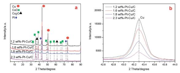
Fig. 1 XRD patterns of 1.2 wt% Pt-Cu/C catalyst, 1.6 wt% Pt-Cu/C catalyst, 1.8 wt% Pt-Cu/C catalyst and 2.3 wt% Pt-Cu/C catalyst (a), magnified Cu characteristic peaks of the four catalysts (b).
