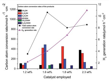
Fig. 9 Carbon conversion rates and  $H_2$  generation rate of  $CO_2$  photoelectrochemical reduction reaction on four catalysts (1.2 wt% Pt-Cu/C catalyst, 1.6 wt% Pt-Cu/C catalyst, 1.8 wt% Pt-Cu/C catalyst, 2.3 wt% Pt-Cu/C catalyst).
