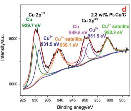
Cu 2p XPS spectra of 1.2 wt% Pt-Cu/C catalyst (a), 1.6 wt% Pt-Cu/C catalyst (b), 1.8 wt% Pt-Cu/C catalyst (c), 2.3 wt% Pt-Cu/C catalyst (d).
