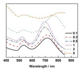
Fig. 2 UV-Vis spectra of the 49 nm Au@Pd@Pt NRs with varied  $\theta_{\rm Pt}$  from 0.1 to 5 layers.
