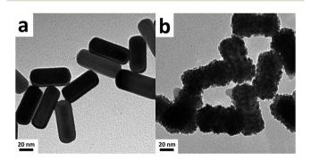
Fig. 1 TEM images of (a) the 49 nm Au NRs and (b) Au@Pd@Pt NRs ( $\theta_{Pt}$  = 5).
