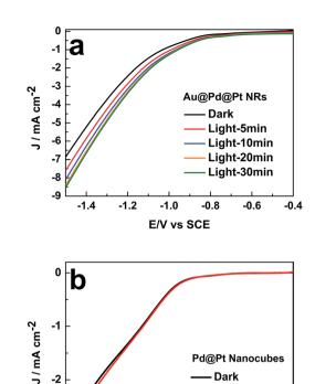
Fig. 4 Influence of the illumination time on the LSV curves of (a) 49 nm Au@Pd@Pt NRs and (b) Pd@Pt nanocubes in  $0.1\,\mathrm{M}$  KHCO $_3$  (pH =  $6.8)~\theta_{\mathrm{Pt}}=0.5$ ; scan rate: 50 mV s $^{-1}$ .
