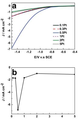
Fig. 3 Influence of  $\theta_{\rm Pt}$  on the LSV curves of (a) 49 nm Au@Pd@Pt NRs measured in 0.1 M KHCO $_3$  (pH = 6.8). Scan rate: 50 mV s $^{-1}$ ; current density of (b) 49 nm Au@Pd@Pt NRs at -1.5 V (vs. SCE) with different  $\theta_{\rm Pt}$ .
