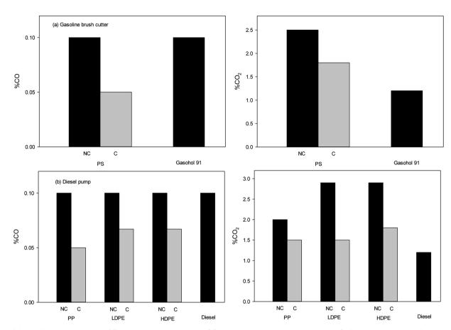
CO and  $CO_2$  emission from (a) gasoline brush cutter and (b) diesel pump at speed of 2000 rpm (NC = no catalyst and C = catalyst)
