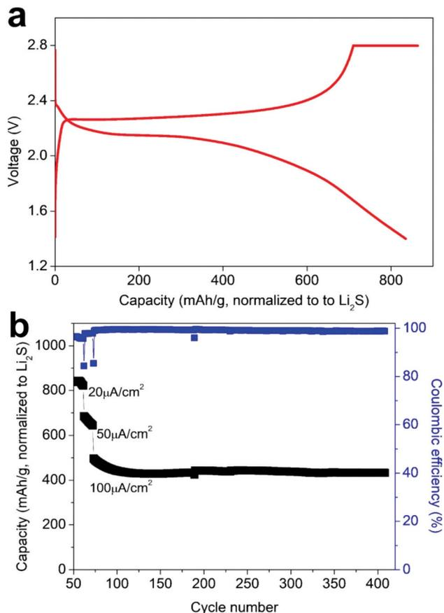
Fig. 4 (a) Typical charge/discharge profile of the all-solid-state battery at 20  $\mu\text{A cm}^{-2}$  current density. (b) Cycle performance of the battery at current densities of 20, 50 and 100  $\mu\text{A cm}^{-2}$  over 400 cycles.
