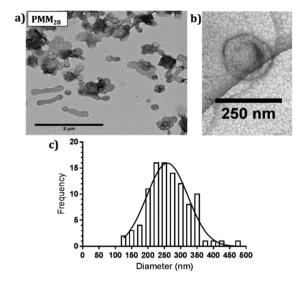
Fig. 3 (a) Negatively stained TEM images of PMM<sub>28</sub> polymersomes, (b) cryo-TEM image of PMM<sub>28</sub> to show hydrated size is consistent with (a). (c) TEM grainsizing of the polymersome sample.
