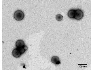
Fig. 4 Unstained TEM images of (a) PMM<sub>28</sub>Fe. The PMM<sub>28</sub> sample was soaked in NaOH (10 mM) before electroporation at 750 V (5 pulses) in the presence of excess FeCl<sub>2</sub>·4H<sub>2</sub>O. The polymersomes show dark electron dense cores, attributed to the precipitation of magnetic iron oxide.
