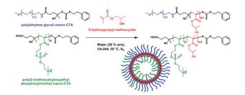
Fig. 2 Poly(ethylene glycol)-poly(2-hydroxypropyl methacrylate)/poly (2-(methacryloyloxy)ethyl phosphorylcholine)-poly(2-hydroxypropyl methacrylate) (PEG + PMPC)-PHPMA polymersomes are prepared by chain extension of a binary mixture of PEG $_{113}$  and PMPC $_{28}$  macro-CTAs via reversible addition–fragmentation chain transfer (RAFT) aqueous dispersion polymerisation of 2-hydroxypropyl methacrylate (HPMA).  $^{45}$
