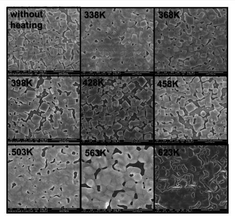
Fig. 4 SEM top view images of CsPbBr<sub>3</sub> thin films at different annealing temperatures. Scale bar is 5 μm.
