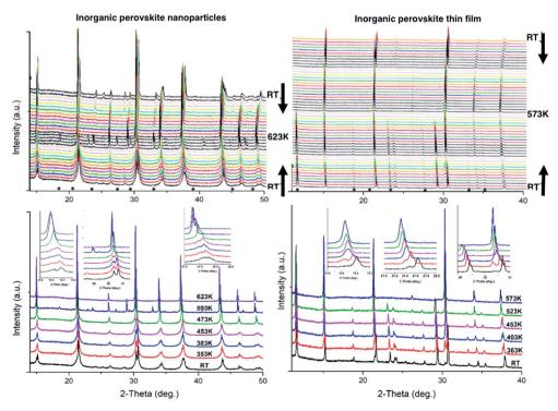
Fig. 1 X-ray diffraction patterns recorded in situ at different temperatures for (left) CsPbBr<sub>3</sub>-based nanoparticles and (right) thin films. Scan step is every 15 K from 308 K to 623 K (top left) and every 10 K in the 303-573 K temperature range (top right) upon cooling and heating. Selected XRD patterns are shown with particular areas in insets. Asterisk symbolizes the CsPb<sub>2</sub>Br<sub>5</sub> phase
