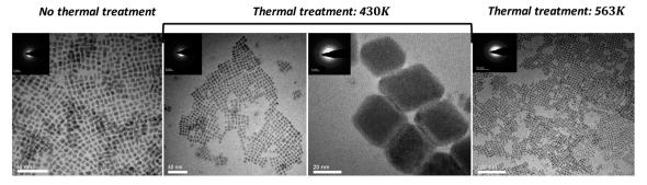
Fig. 5 TEM micrographs of CsPbBr<sub>3</sub> and CsPb<sub>2</sub>Br<sub>5</sub> NPs after different annealing temperatures. Insets correspond to the electron diffraction patterns taken from these NPs.
