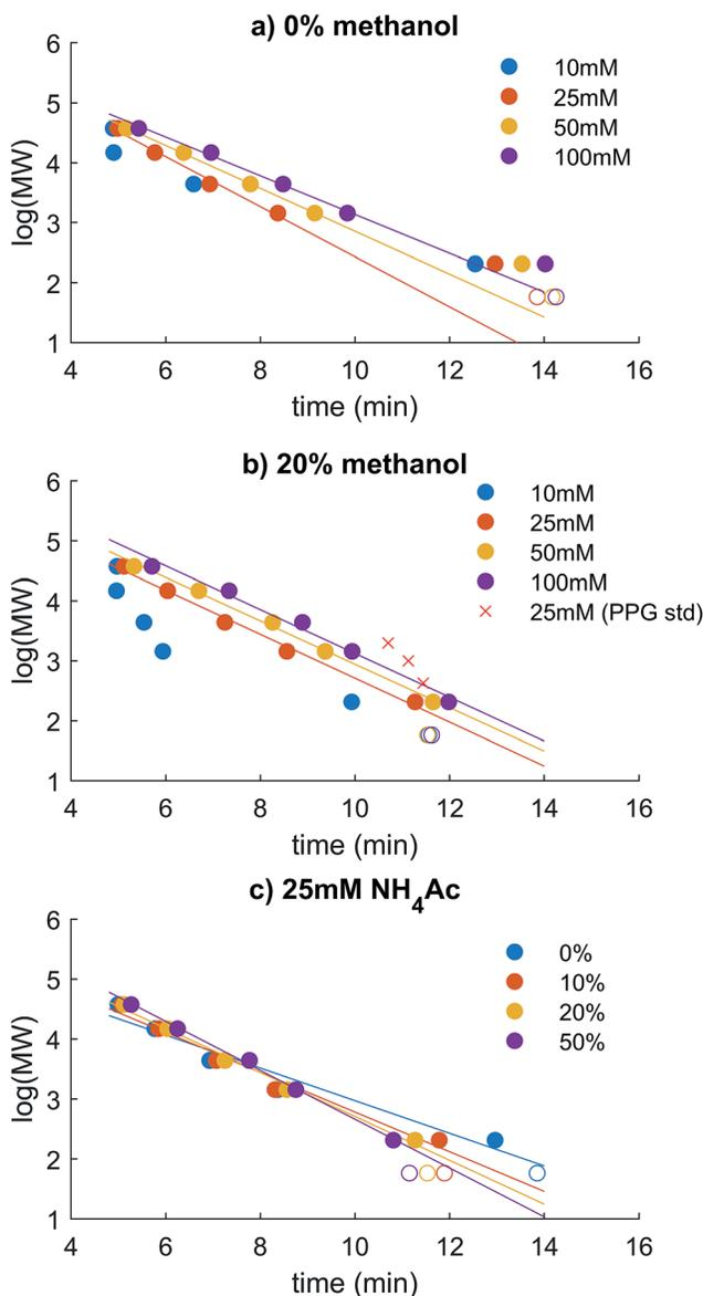
Fig. 1  $\log(MW)$  vs. retention time relationship of PSS standards (filled circles) in various mobile phases. Note the variation in retention time of acetone, plotted as an unfilled circle. Polypropylene glycol (PPG) standards are plotted as red crosses. (a–c) Different mobile phase conditions, as indicated by the titles and legends.
