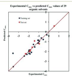
Fig. 12 The scatter plot of the observed and the predicted dispersibility index of SWCNTs ( $\log C_{\text{max}}$ ) of the developed PLS model (model P1).
