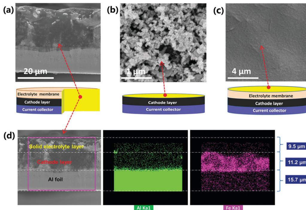
Fig. 3 (a) SEM image of the cross section of the cathode-supported PPAL solid electrolyte membrane. (b) Surface morphology of the  $\text{LiFePO}_4$  cathode layer. (c) Surface morphology of the PPAL solid electrolyte membrane. (d) EDS maps of Al and Fe in the cross section of the cathode-supported PPAL solid electrolyte membrane.
