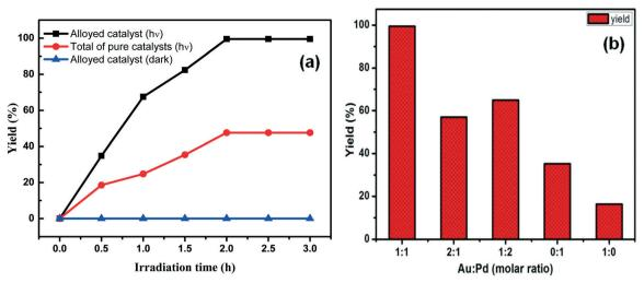
Fig. 7 Biphenyl yield (a) using different spatial arrangements of catalyst and (b) depending on the metal ratio of Au: Pd.
