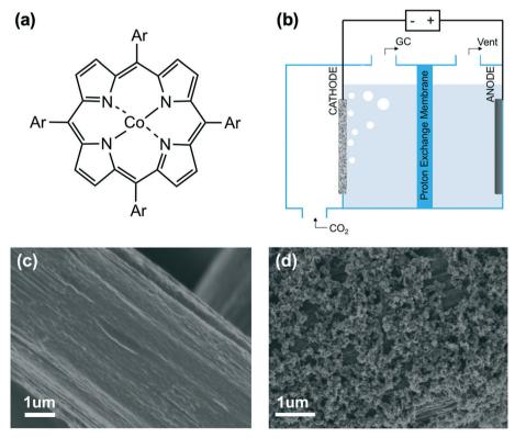
Fig. 1 (a) Chemical structure of cobalt porphyrin with aromatic substituents (Ar). (b) Schematic of three-compartment cell configuration. (c) SEM image of pristine carbon paper. (d) SEM image of electrode with CoTPP catalyst at a loading of  $1 \times 10^{-8}$  mol cm<sup>-2</sup>
