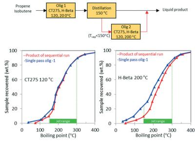
Fig. 11 Simulated distillation results for the reaction product of model isobutene/propene (4/1 molar) feed mixture over H-beta (left figure) and CT275 (right figure) after single-pass conversion (blue line) and after a second oligomerization (red line) of the light olefins obtained in the first run (b.p. < 150 °C).
