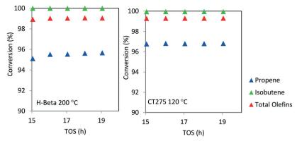
Fig. 7 Isobutene/propene conversion over H-beta (200 °C) and CT275 (120 °C) catalysts (4:1 molar ratio, p = 1.38 MPa, WHSV = 1.1 h<sup>-1</sup>).
