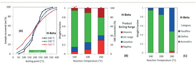
Fig. 4 (A) Simulated distillation and GC-MS analysis for the liquids products derived from DIB feed reaction over H-beta zeolite as classified by (B) by boiling-point range and (C) chemical functionality. DIB (b.p. 101 °C) is fully converted to a wide boiling mixture of hydrocarbons.
