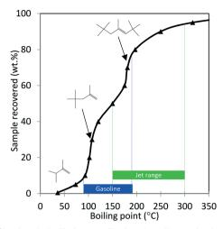
Fig. 9 Simulated distillation profile for the oligomerization product shown in Table 4 collected after 350 hours TOS (Amberlyst-36 catalyst; p = 1.38 MPa, 140 °C, WHSV = 1.1 h<sup>-1</sup>). Proposed structures of major products with corresponding boiling points were obtained from GC-MS analysis.
