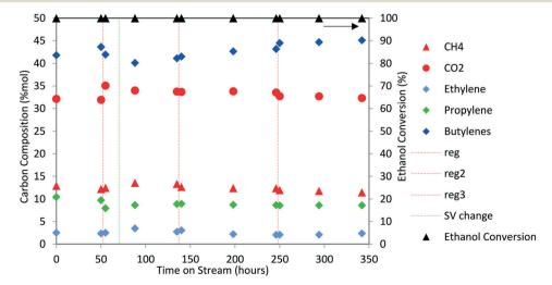
Fig. 8 Ethanol conversion (mol%) and product selectivity (mol C%) over Zn<sub>1</sub>Zr<sub>2.5</sub>O<sub>z</sub> (50 wt% ethanol in water feed; 450 °C, 1.38 MPa, GHSV = 320 to 660  $h^{-1}$ ). Vertical red dotted lines represent regeneration steps and green dotted line marks a change in contact time.
