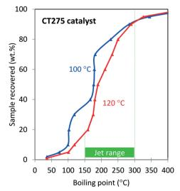
Fig. 6 Effect of oligomerization temperature on simulated distillation profiles for the oligomerization product of a model isobutene/propene model feed over CT275 catalyst (4:1 molar ratio; 3 hours TOS, p = 1.38 MPa, WHSV =  $1.1 h^{-1}$ ).
