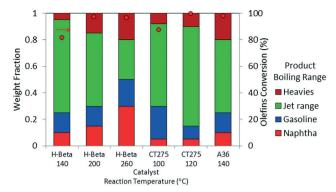
Fig. 5 Product yields based on simulated distillation for the oligomerization liquid product of model isobutene/propene (4:1 molar ratio; 3 hours TOS, p = 1.38 MPa, WHSV =  $1.1 \text{ h}^{-1}$ ).
