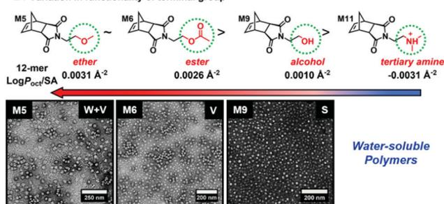
**Fig. 2** Oligomer  $\log P_{oct}/SA$  values as a function of (A) anchor and (B) terminal group variations for NB-based monomers suitable for use as core-forming blocks during aqueous ROMPISA, and representative nano-object TEM images for corresponding diblock copolymers of approximately the same length. Adapted with permission from ref. 59. Copyright 2019 American Chemical Society.
