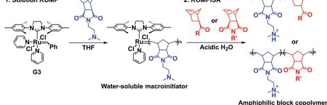
**Scheme 2** Reported synthetic strategies to conduct aqueous dispersion ROMPISA for fabrication of diblock copolymer nano-objects of various morphologies. (A) One-pot aqueous ROMPISA mediated by a water-soluble **HG2** catalyst, and (B) two-step aqueous ROMPISA mediated *via* a water-soluble PNB macroinitiator prepared in organic solvent using **G3**.
