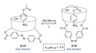
Scheme 7 Photocontrol over ester hydrolysis catalysed by azobenzenecapped β-cyclodextrin 15.
