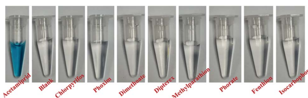
Fig. 4 Selectivity tests of the visual detection method for acetamiprid against other pesticides. The concentration is 10 nM for acetamiprid and 100 nM for other control molecules.
