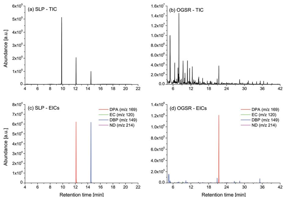
**Fig. 2** Comparison of total ion chromatograms (TICs) and overlaid extracted ion chromatograms (EICs) for selected compounds (*i.e.*, DPA, EC, DBP, 2ND and 4ND) between a SLP analysed by SE-GC-MS and its respective OGSR analysed by HSSE-TD-GC-MS. Ammunition was a Sellier & Bellot .357 Magnum. Noteworthy are the significant differences in the ratios of the selected compounds.
