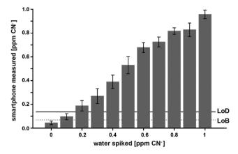
Fig. 5 Results of the cyanide-spiked H<sub>2</sub>O samples that were analysed with the smartphone app (12 measurements for each concentration). The limit of blank (LoB) and the limit of detection (LoD) are represented as dotted and continuous lines, respectively.
