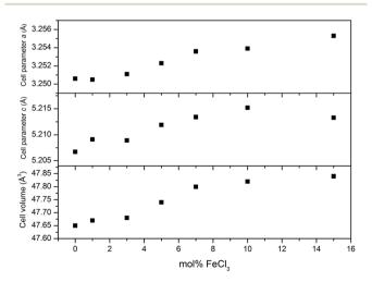
Fig. 5 Variation of cell parameters a, c and cell volume of the films with a change of mol% FeCl<sub>3</sub> added to the precursor solution. The increase of cell parameters confirms the incorporation of Cl into the ZnO lattice.
