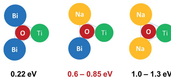
Fig. 3 Saddle-point configuration and associated activation energies for oxygen ion migration in NBT. Values taken from ref. 37.
