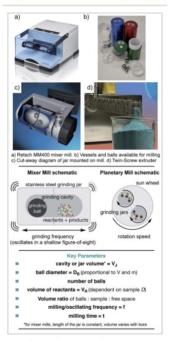
Scheme 1 Examples of equipment used for mechanochemical reactions and key parameters. (a & c) Reproduced with permission from Retsch, (b) reproduced with permission from FormTech Scientific. (d) Reproduced with permission from Prof Stuart James and RSC.
