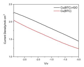
Fig. 7 J-V curves of Cu(BTC)-rGO catalyst and Cu(BTC) catalyst obtained from CO<sub>2</sub> electrochemical reduction in DMF (three electrode configuration, without photoanode).
