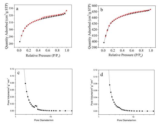
Nitrogen sorption isotherms: Cu(BTC)-rGO (a), Cu(BTC) (b); pore size distribution: Cu(BTC)-rGO (c), Cu(BTC) (d).
