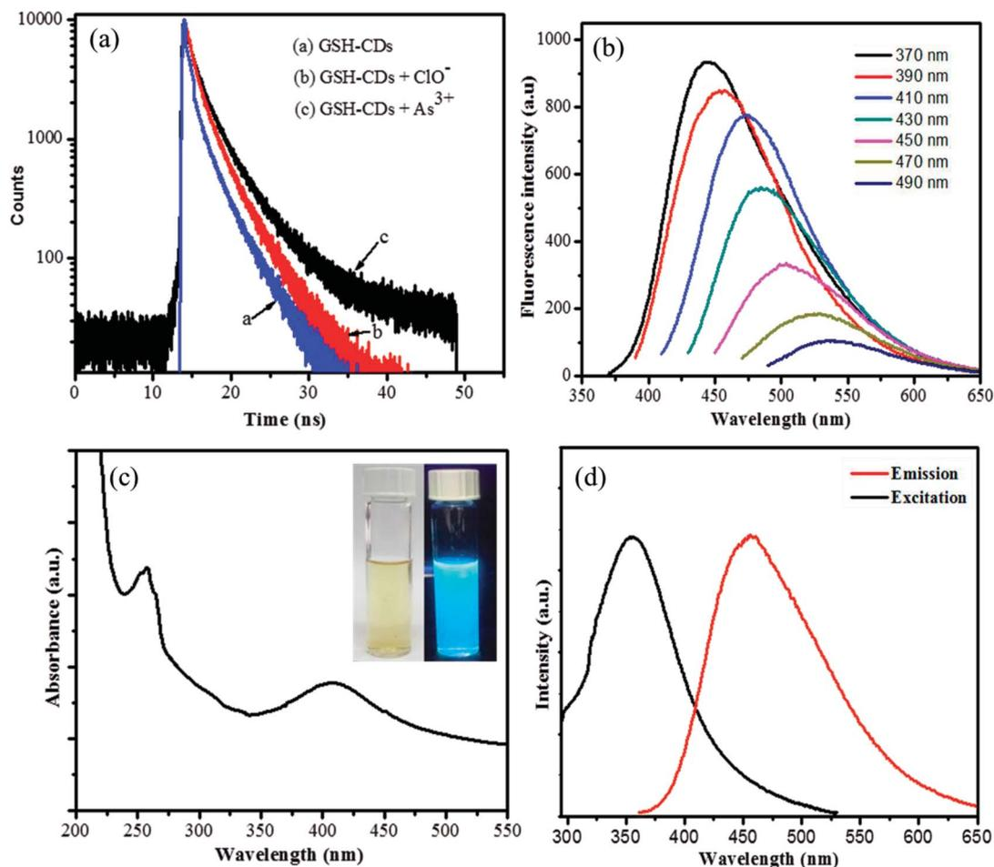
Fig. 5 (a) Fluorescence decay curves of GSH-CDs (blue colored curve (a)), GSH-CDs with  $\text{ClO}^-$  (red colored curve (b)), and GSH-CDs with  $\text{As}^{3+}$  (black colored curve (c)). (b) Excitation-dependent fluorescence emission of GSH-CDs with excitation from 370 to 490 nm. (c) UV-vis absorption spectra of GSH-CDs. The inset image is an aqueous dispersion of GSH-CDs in day light and UV light, respectively. (d) Fluorescence excitation and emission response of the GSH-CDs.
