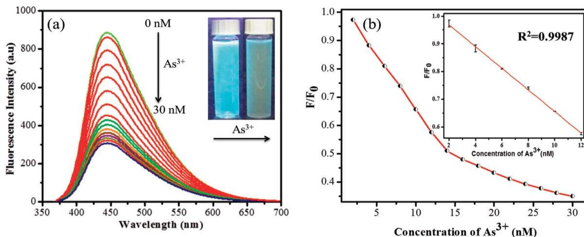
Fig. 7 (a) Fluorescence emission response of 10  $\mu\text{L}$  GSH-CDs, to various molar equivalents of  $\text{As}^{3+}$  ions (0 to 30 nM) in 1000  $\mu\text{L}$  of tris–HAc buffer (10 mM, pH 7.4). (b) Stern–Volmer plot with an inset plot shows the linearity for  $\text{As}^{3+}$  ions (2 to 12 nM).
