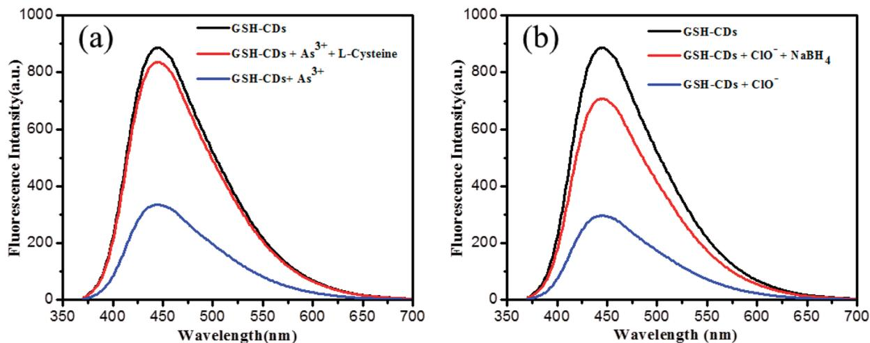
Fig. 11 (a) Fluorescence response 10  $\mu\text{L}$  of GSH-CDs for  $\text{As}^{3+}$  ions (25 nM) and recovery of L-cysteine. (b) Fluorescence response of GSH-CDs for  $\text{ClO}^-$  ions (100  $\mu\text{M}$ ) and the recovery of  $\text{NaBH}_4$ .
