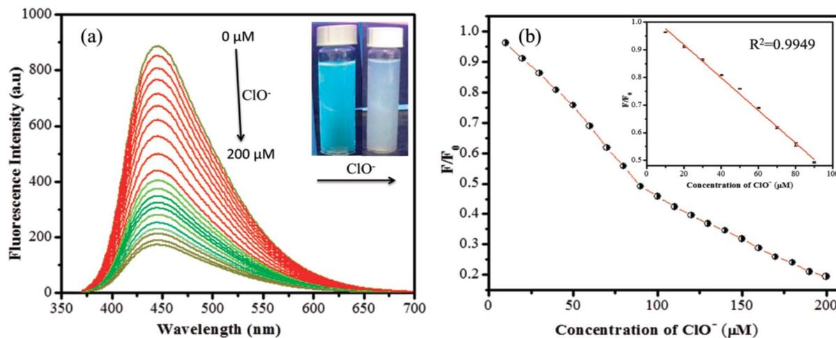
Fig. 8 (a) Fluorescence emission response of 10  $\mu\text{L}$  GSH-CDs, to various molar equivalents of  $\text{ClO}^-$  ions (0 to 200  $\mu\text{M}$ ) in 1000  $\mu\text{L}$  of tris-HAc buffer (10 mM, pH 7.4). (b) Stern-Volmer plot shows the linearity for  $\text{ClO}^-$  ions (10 to 90  $\mu\text{M}$ ).
