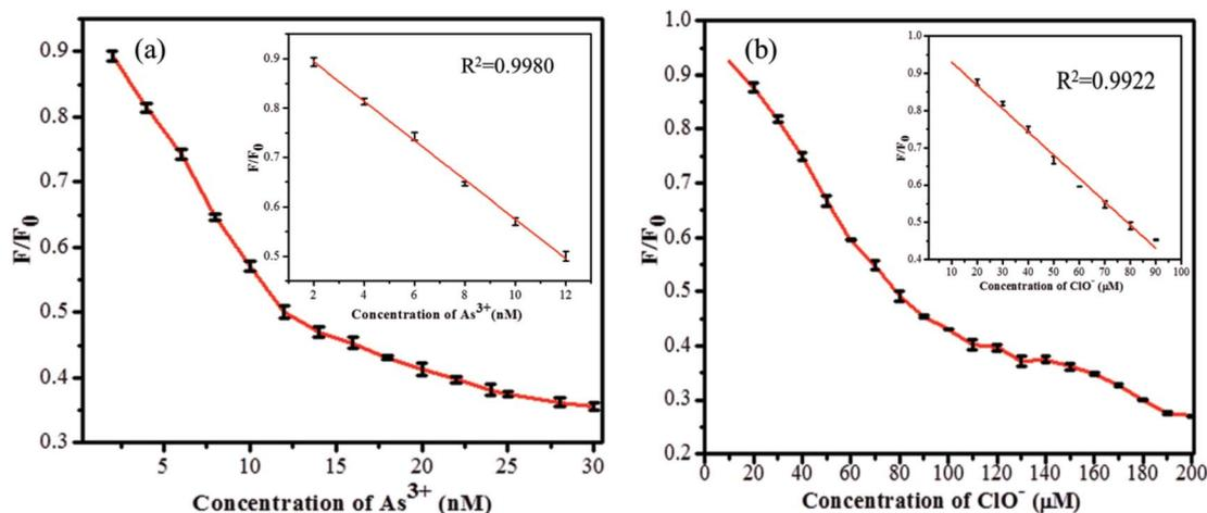
Fig. 12 (a) Fluorescence response of GSH-CDs for  $\text{As}^{3+}$  ions (0–30 nM) in tap water, (b) for  $\text{ClO}^-$  ions (0–200  $\mu\text{M}$ ) in tap water. The triplicated data were fitted in the linearity equation of  $F_0/F$  for tap water sample analysis, shown as in insert image.
