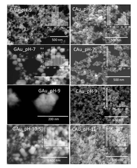
Fig. 2 Typical SEM images of GAuNPs (left column) and CAuNPs (right column) synthesized at different pH values of the reaction mixture. Insets show histogram reflecting the size dispersion corresponding to each pH; average size of the NPs vs. number of particles.
