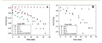
Fig. 8 Kinetics of 4-NP degradation by (A) GAuNPs, and (B) and CAuNPs fabricated at different pH values of reaction mixtures.
