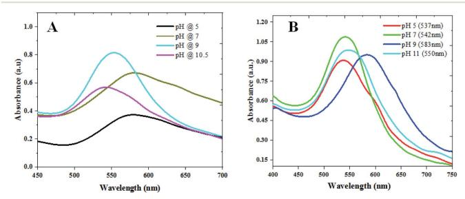
Fig. 1 Absorbance spectra of the colloidal (A) GAuNPs and (B) CAuNPs synthesized at different pH values of the reaction mixtures.
