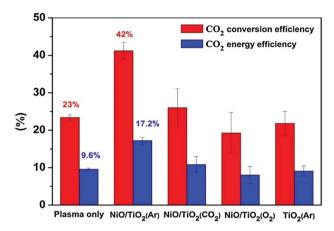
Fig. 5  $CO_2$  conversion and energy efficiencies, measured during the plasma-catalysis  $CO_2$  dissociation, are shown for the NiO/TiO<sub>2</sub> catalysts prepared by plasma treatment with different gases (O<sub>2</sub>, Ar, CO<sub>2</sub>). Reproduced from ref. 198 with permission from Elsevier, copyright 2016.
