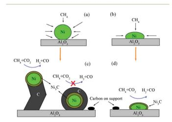
Fig. 3 Schematic representation of CO<sub>2</sub>/CH<sub>4</sub> reforming over (a and c) NiAl-C (calcinated); and (b and d) NiAl-PC (plasma treated prior to calcination) samples. Reproduced from ref. 161 with permission from Elsevier, copyright 2008.
