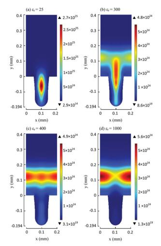
Fig. 8 Distributions of the electron impact ionization rate, averaged over time in one AC cycle, for different dielectric constants: (a)  $\varepsilon_r = 25$ , (b)  $\varepsilon_{\rm r}=300$ , (c)  $\varepsilon_{\rm r}=400$ , and (d)  $\varepsilon_{\rm r}=1000$ , for a helium discharge sustained at 20 kV with a 100 µm pore. Reproduced from ref. 223 with permission from American Chemical Society, copyright 2016.
