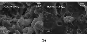
Fig. 8 Comparative (a) PXRD patterns and (b) SEM images taken on fresh and used H\_Ru10-GDEs ( $t_0$ ,  $t_{45}$  and  $t_{300}$  stand for GDEs subjected to 0, 45 and 300 min).
