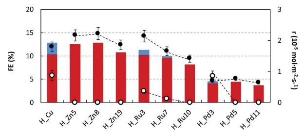
Fig. 7 FEs for C<sub>2</sub>H<sub>5</sub>OH (in red) and CH<sub>3</sub>OH (in blue) formation and r for C<sub>2</sub>H<sub>5</sub>OH (•) and CH<sub>3</sub>OH (•) in the electrocatalytic reduction of CO<sub>2</sub> at H\_Zn, H\_Ru and H\_Pd in comparison to H\_Cu.
