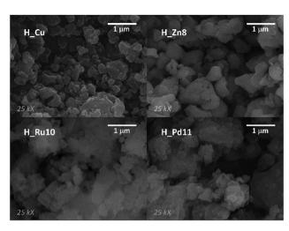
Fig. 2 SEM micrographs (SEI mode) at 25 000 magnifications of H\_Cu, H\_Zn8, H\_Ru10, and H\_Pd11.
