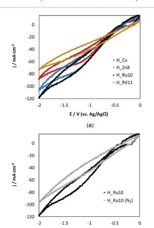
Fig. 5 Cyclic-voltammetry responses for (a)  $H_Zn8$ ,  $H_Ru10$  and  $H_Pd11$  in comparison to  $H_Cu$ -based GDEs in a medium saturated with  $CO_2$  and, (b) responses for  $H_Ru10$  in the presence and absence of  $CO_2$ .
