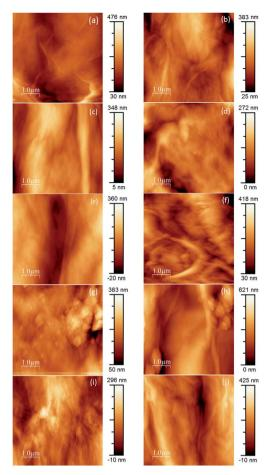
Fig. 10 AFM images of pristine and amine-functionalized GOP samples. Pristine GOP (a and b), GOP-AP (c and d), GOP-DAN (e and f), GO-ODA (g and h) and GOP-DAD (i and j). The left column (a, c, e, g, i) shows the lower mat side which was in contact with the filter membrane during GOP fabrication; the right column (b, d, f, h, j), to the upper mat side.
