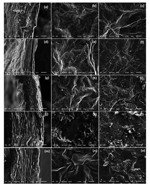
Fig. 8 Representative SEM images of pristine GOP (a-c), GOP-AP (d-f), GOP-DAN (g-i), GO-ODA (j-l) and GOP-DAD (m-o). The left column (a, d, g, j, m) shows cross-section images; the middle column (b, e, h, k, n) corresponds to the upper mat side; the right column (c, f, i, l, o), to the lower mat side which was in contact with the filter membrane during GOP fabrication. Scale bar, 5 µm in all images.
