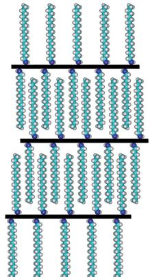
Fig. 9 Schematic representation of the mechanism of GO nanosheet ordering in GOP-ODA.
