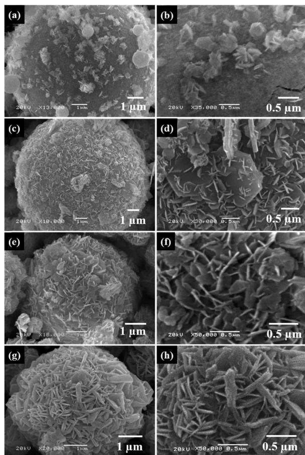
Fig. 4 SEM of the  $\text{Ni}_{0.8}\text{Co}_{0.1}\text{Mn}_{0.1}(\text{OH})_2@ \text{Ni}_{0.8}\text{Co}_{0.1}\text{Mn}_{0.1}\text{O}_x$  precursor obtained at different time intervals during the co-precipitation reaction: (a and b)  $0.5 \text{ h}$ ; (c and d)  $1 \text{ h}$ ; (e and f)  $1.5 \text{ h}$ ; (g and h)  $2 \text{ h}$ .
