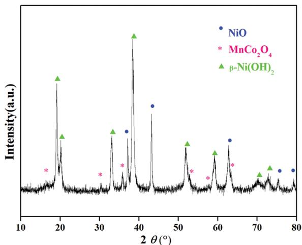
Fig. 1 XRD patterns of the  $\text{Ni}_{0.8}\text{Co}_{0.1}\text{Mn}_{0.1}(\text{OH})_2@ \text{Ni}_{0.8}\text{Co}_{0.1}\text{Mn}_{0.1}\text{O}_x$  precursor.
