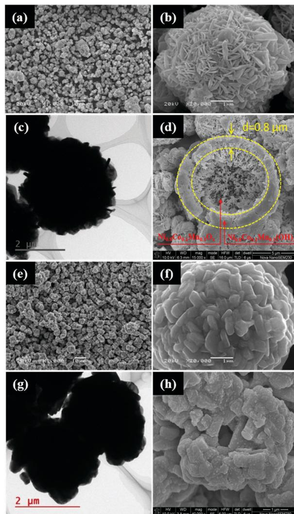
Fig. 3 (a) Low-magnification SEM, (b) high-magnification SEM, (c) TEM and (d) cross-sectional SEM images of the holistic  $\text{Ni}_{0.8}\text{Co}_{0.1}\text{Mn}_{0.1}(\text{OH})_2@ \text{Ni}_{0.8}\text{Co}_{0.1}\text{Mn}_{0.1}\text{O}_x$  precursor. (e) Low-magnification SEM, (f) high-magnification SEM, (g) TEM and (h) cross-sectional SEM images of the  $\text{LiNi}_{0.8}\text{Co}_{0.1}\text{Mn}_{0.1}\text{O}_2$  microspheres.
