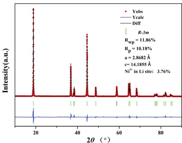
Fig. 2 Rietveld refinement profile of the XRD data of the  $\text{LiNi}_{0.8}\text{Co}_{0.1}\text{Mn}_{0.1}\text{O}_2$  cathode prepared from  $\text{Ni}_{0.8}\text{Co}_{0.1}\text{Mn}_{0.1}(\text{OH})_2@ \text{Ni}_{0.8}\text{Co}_{0.1}\text{Mn}_{0.1}\text{O}_x$ .
