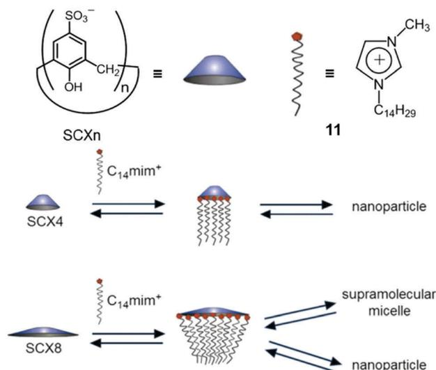
Fig. 9 Schematic representation of different self-assemblies formed by different *p*-sulfonatocalix[*n*]arenes (SCX*n*, *n* = 4 or 8). Adapted with permission from ref. 53. Copyright 2017 American Chemical Society.
