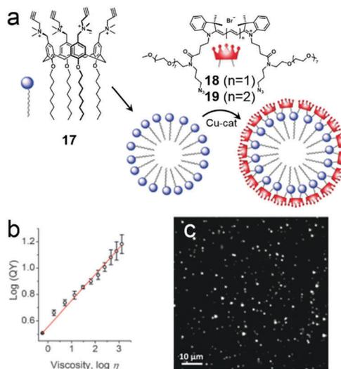
**Fig. 12** (a) Chemical structures of amphiphilic calixarene **17** and cyanine dyes (**18** and **19**) and a schematic representation of the formation of the micelles. (b) Dependence of the fluorescent quantum yield on viscosity. (c) Wide-field fluorescence image of **18** coated NPs deposited on glass. Adapted with permission from ref. 64. Copyright 2016 John Wiley and Sons.
