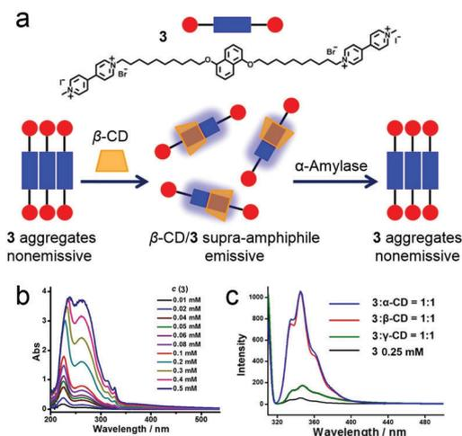
Fig. 4 (a) Schematic representation of the enzyme-responsive supra-amphiphile. (b) UV-vis spectra of **3** with varying concentration. (c) Fluorescence spectra of **3** before and after adding cyclodextrins. Adapted with permission from ref. 31. Copyright 2016 American Chemical Society.
