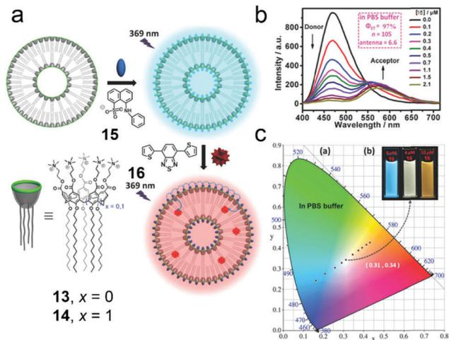
**Fig. 11** (a) Schematic representation of the formation of the broad-spectrum tunable photoluminescent materials. (b) Fluorescence spectra of the **14/15** assembly in PBS buffer with different concentrations of **16**,  $\lambda_{ex} = 369$  nm. (c) The luminescent color changes of the **14/15** assembly with different concentrations of **16** in PBS buffer. Adapted with permission from ref. 62. Copyright 2016 John Wiley and Sons.
