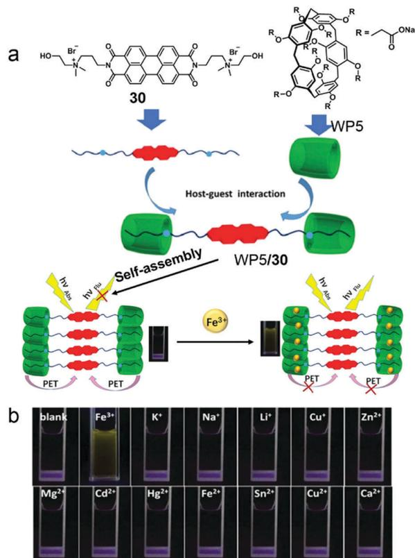
Fig. 23 (a) Chemical structures of the host and guest compounds and a cartoon representation of the  $\text{Fe}^{3+}$  ion sensing mechanism. (b) Photographs of WP5/30 supra-amphiphile solutions after adding various metal ions under UV light. Adapted with permission from ref. 95. Copyright 2017 American Chemical Society.
