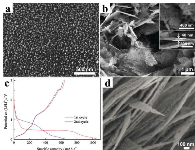
**Fig. 3** (a) SEM image of the as-deposited ZnO at  $500^\circ\text{C}$ . Reproduced with permission.<sup>44</sup> Copyright 2003, The Electrochemical Society. (b) SEM image of mesoporous ZnO nanosheets; (c) the first two charging/discharging curves of mesoporous ZnO nanosheets. Reproduced with permission.<sup>45</sup> Copyright 2014, Elsevier. (d) SEM image of the ZnO nanosheets. Reproduced with permission.<sup>46</sup> Copyright 2016, Springer.
