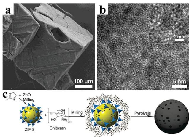
Fig. 7 (a) SEM image and (b) TEM image of ZnO QDs@porous carbon. Reproduced with permission.<sup>93</sup> Copyright 2013, American Chemical Society. (c) Synthetic route of ZIF-8@chitosan-800N. Reproduced with permission.<sup>94</sup> Copyright 2014, Royal Society of Chemistry.
