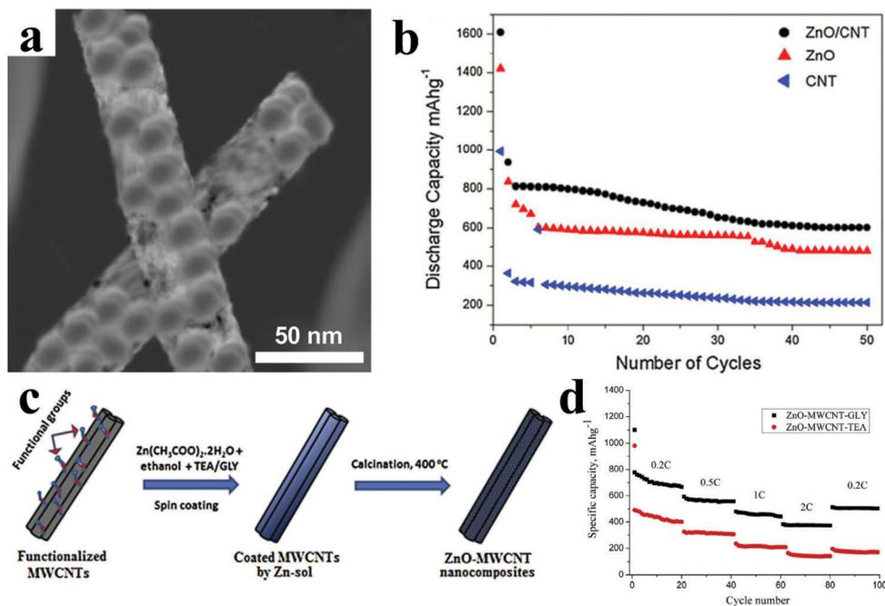
Fig. 6 (a) TEM image of ZnO/CNT composites; (b) cycling performances of bare CNTs, ZnO, and ZnO/CNT electrodes. Reproduced with permission.<sup>79</sup> Copyright 2013, Springer. (c) Schematic illustration of facile sol-gel synthesis of nanocomposite anodes; (d) the rate capabilities of the ZnO/MWCNT buckypaper nanocomposite anodes. Reproduced with permission.<sup>81</sup> Copyright 2015, Elsevier.
