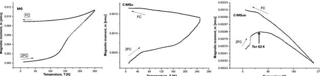
Fig. 6 Thermomagnetic curves (temperature dependence of magnetization measured using the standard zero field cooling (ZFC) and field cooling (FC) procedure) for MG, C-MGst, C-MGultr.
