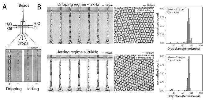
Fig. 3 Bead-dependent drop formation in the jetting regime with an aqueous co-flow. A) Device schematic with fluid inlets and outlets. Device operation in the dripping and jetting regimes with and without 50 µm beads. B) Frames from a video of device operation in the dripping (top) and jetting (bottom) regimes. The resultant emulsions and drop diameter histograms are shown to the right of time lapse images.
