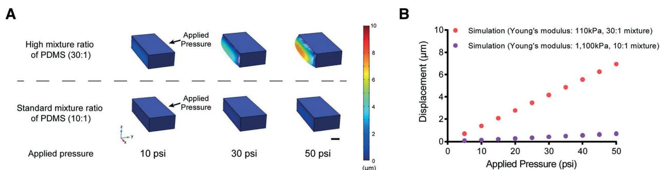
**Fig. 2** Simulation results for the displacement of the actuated membrane by applying various pressures. (A) Examples of PDMS membrane deformation using different applied pressures from the results of COMSOL simulation. The color bar represents the scale of membrane displacement. Scale bar: 10 μm. (B) Red and purple represent simulation results from COMSOL Multiphysics (Young's modulus – red (30:1 PDMS mixture used in this study: 110 kPa) and purple (10:1 standard PDMS mixture: 1100 kPa)).
