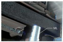
Fig. 7 Inline measurement of steel blooms, left: the bloom is transported on a roller table and arriving from the left, right: the measuring lance (ML) is approached to the side face of the bloom, laser irradiation is activated to locally ablate the scale layer and to analyse the bulk composition. Diameter of ML: 170 mm.<sup>32</sup>
