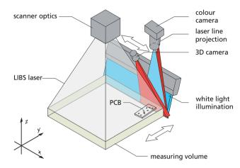
Fig. 11 Principal set-up of machine II of the ADIR demonstrator.
