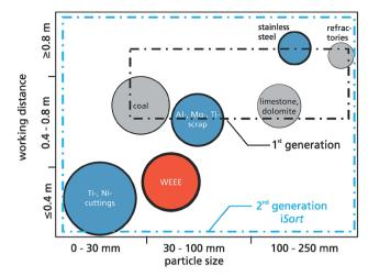
Fig. 3 Application fields of inline monitoring and identification tasks by LIBS on moving objects illustrated in the coordinates working distance versus particle size. WEEE = waste electric and electronic equipment. The dashed rectangles indicate the working range of 1<sup>st</sup> and 2<sup>nd</sup> generation LIBS machines, cf. Table 1. Filling-in colours are assigned as follows: blue = metals, grey = non-conductive materials, red = mixture of metals and non-metals.
