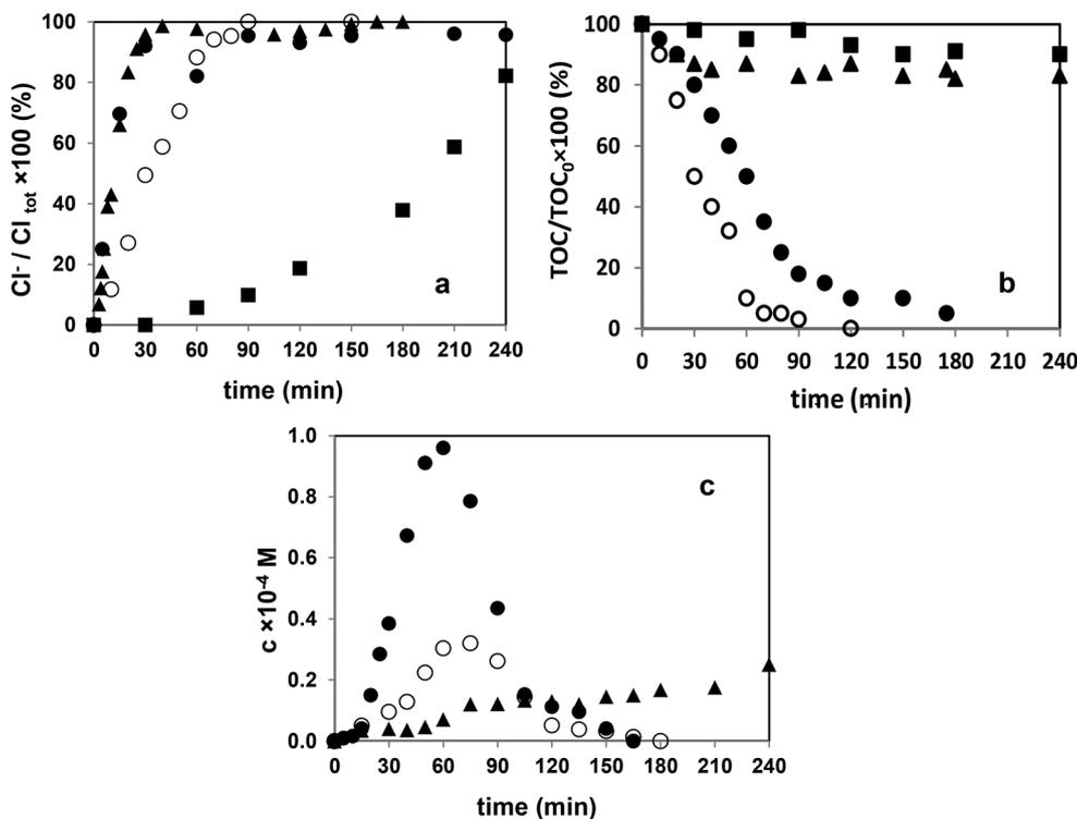
**Fig. 5** Relative concentration of  $\text{Cl}^-$  (a), total organic carbon content (TOC) (b) and sum of the concentration of peroxides ( $\text{H}_2\text{O}_2$ , methyl- and ethyl-hydroperoxides) (c) in the case of the transformation of diuron in aerated solutions/suspension ■: ozonation; ▲: UV photolysis; ●: combination of UV photolysis with ozonation; ○: heterogeneous photocatalysis.
