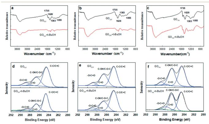
Fig. 4 FTIR spectra of (a) GO<sub>full</sub>, GO<sub>full</sub> with quenching (using t-BuOH) (b) GO<sub>UV</sub>, GO<sub>UV</sub> with t-BuOH and (c) GO<sub>vis</sub>, GO<sub>vis</sub> with t-BuOH; XPS spectra of (d)  $GO_{tull}$ ,  $GO_{tull}$  with quenching (t-BuOH) (e)  $GO_{UV}$ ,  $GO_{UV}$  with t-BuOH and (f)  $GO_{vis}$ ,  $GO_{vis}$  with t-BuOH.
