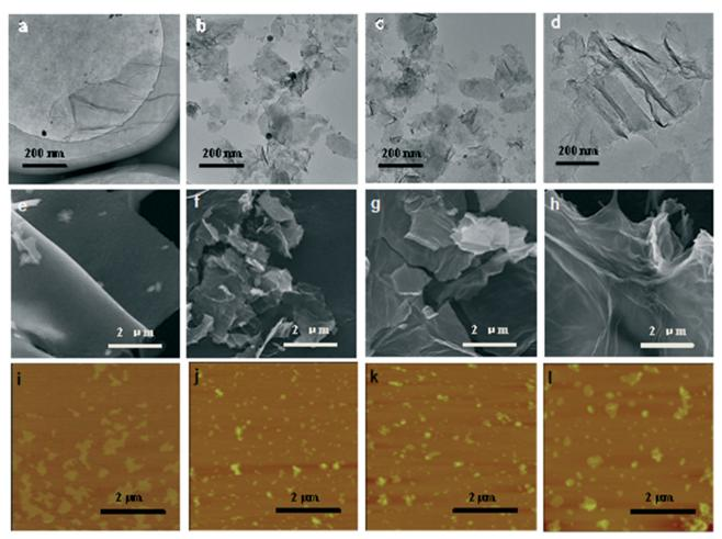
Fig. 2 TEM micrographs of (a) pristine GO, (b) GO<sub>full</sub>, (c) GO<sub>UV</sub>, and (d) GO<sub>vis</sub>. SEM micrographs of (e) pristine GO, (f) GO<sub>full</sub>, (g) GO<sub>UV</sub>, and (h)  $GO_{vis}$ . AFM images of (i) pristine GO, (j)  $GO_{full}$ , (k)  $GO_{UV}$ , and (l)  $GO_{vis}$ . The irradiation time was 24 h for all the samples.
