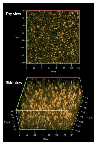
Fig. 2 142.86  $\mu$ m  $\times$  142.86  $\mu$ m CLSM 64  $\mu$ m Z-stack image of CdSe/ ZnS-PMMA polymer nanocomposite obtained with 458 nm excitation. Any emission detected above a 505 nm cut-off filter is shown in orange, which includes the QD  $\lambda_{max}$  = 594 nm.
